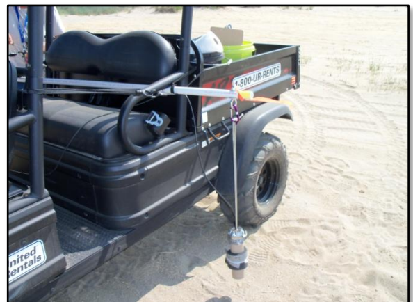
GPS Gamma Ray Survey Unit mounted on ATV.
